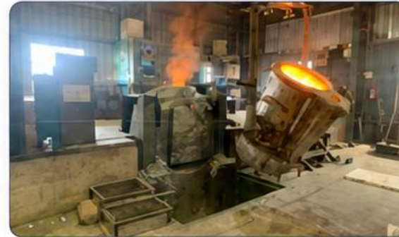
INDUCTION FURNACE 500 kW, 500 Kg
