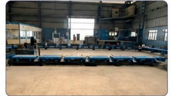
HYDRAULIC LOOP LINE 32 Pallet
