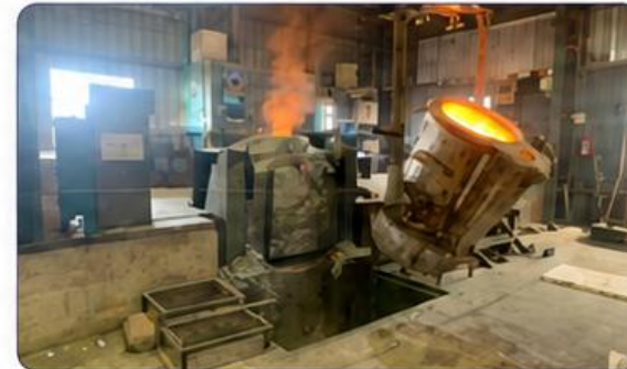
INDUCTION FURNACE 500 kW, 500 Kg
